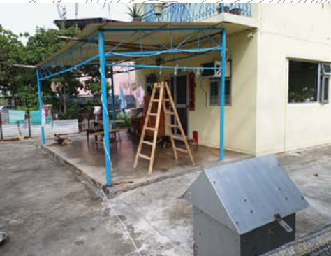
HVS placed inside premises of San Uk Ling Village House No.1 during baseline air quality monitoring
